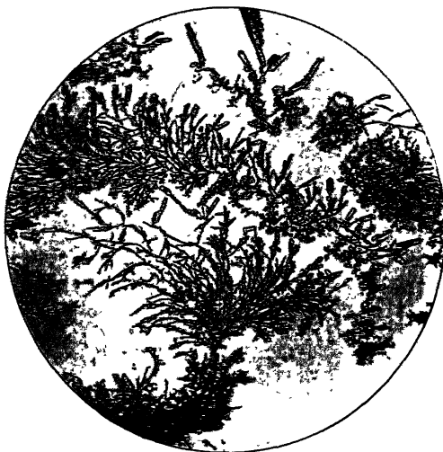
FIG. 49.—Potassium Bichromate rapidly crystallised from a Labile Solution
